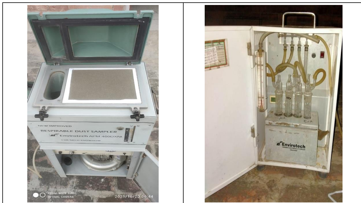
Figure 1: Respirable Dust Sampler for Sampling of PM 2.5, SO 2 and NO 2
