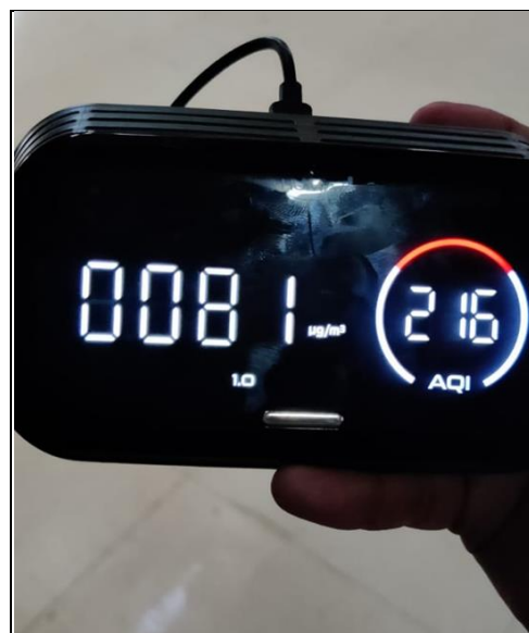
Figure 6: Portable Air Quality Monitor Reading of PM 1 and AQI at Bhai Gurdas Library, GNDU, Campus.
